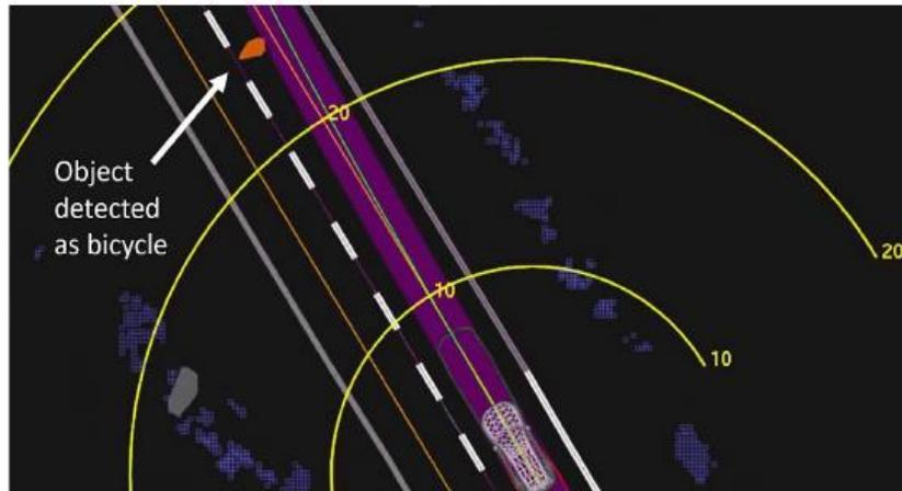
*Figure from the US National Transportation Safety Board Preliminary Report (May 2018) showing the video of the self-driving system data playback approx. 1.3 seconds before impact.*
